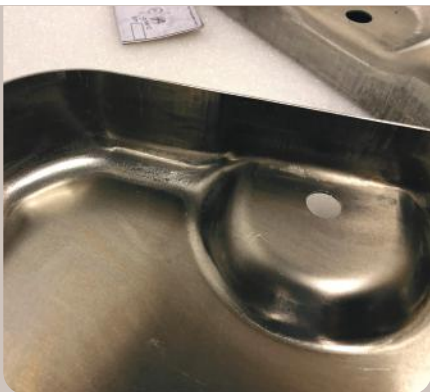
Press forming the high-tensile aluminium sheets using a 200 ton power press, followed by trimming using a 5-axis laser cutter
