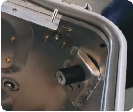
Panel ring with EMC oriented wires gasket in silicone
