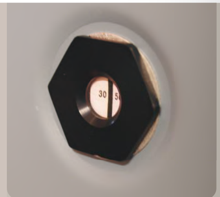
Humidity indicator showing various RH levels
